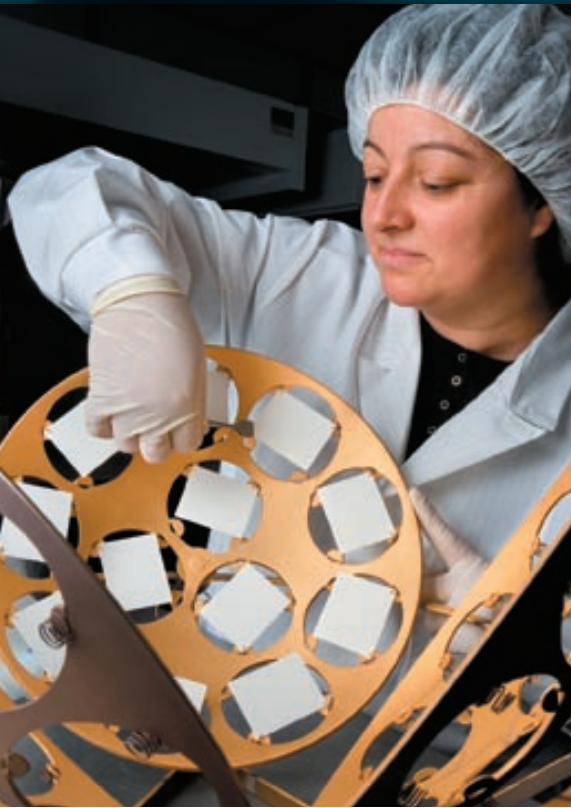
An employee of Stellar Industries in Millbury, Mass., readies beryllia ceramic plates from Brush Ceramic Products for metal deposition. After metalization, Stellar will produce laser diode submounts from these materials. (below center)
